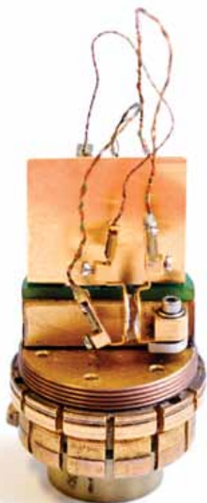
Mary Anne White in a DREAMS laboratory at Dalhousie University. She is holding a sample holder (right) from the Physical Property Measurement System (PPMS) that is used to measure thermal and electrical resistance.
